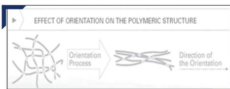
Biaxially Oriented PVC Pipes were discovered many years ago, and the most common application is potable water distribution under pressure. Molecular orientation results in an exceptionally tough, high performance thermoplastic pipe with greatly enhanced physical and mechanical characteristics, increased hydraulic capacity, greater impact resistance, higher strength, elasticity & ductility, improved
